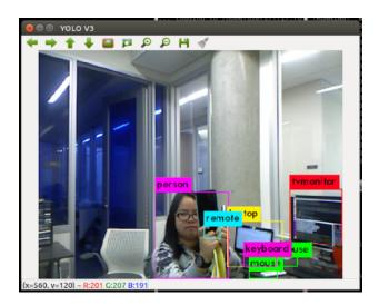
Fig. 1. An example of YOLO working with input from the Microsoft Xbox Kinect in a indoor setting. It recognizes most objects from its databases and then publishes bounding boxes around them.
